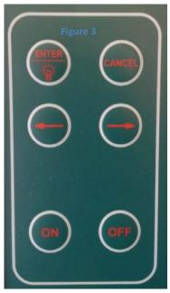
The keypad with six buttons (Fig. 3) is on the same panel and located between the LCD and the cuvette compartment. The keypad controls are responsible for the use of the following functions:
